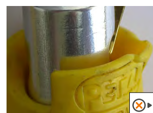
• Defective locking system
