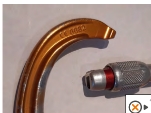
• Defective return spring
