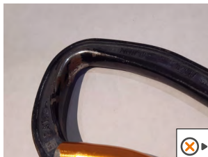
• Frame worn by the rope
