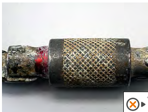
• Defective locking system
