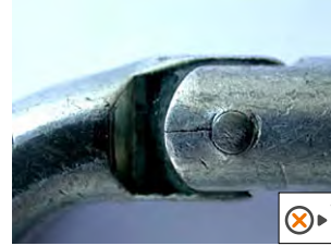
• Broken locking sleeve
