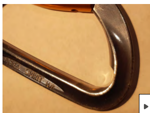
• Defective return spring
