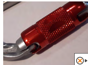
• Defective locking system
