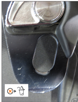
• Attachment hole deformed by a shock load
