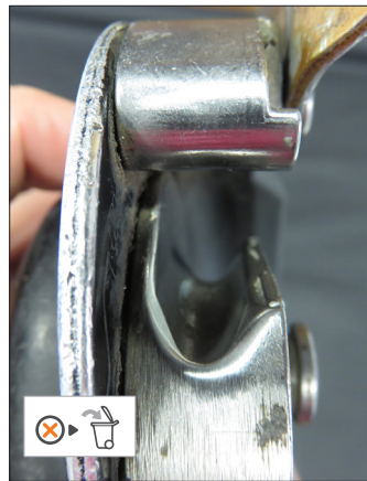
• Cam groove worn to wear indicator
