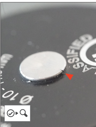
• Rivet slightly cracked
